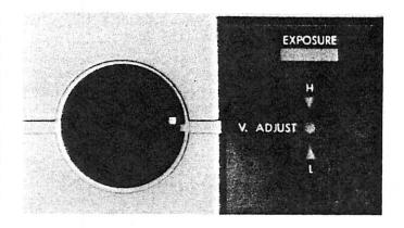
Note: The x-ray unit will not make an exposure unless the green operating voltage indicating lamp is illuminated.
